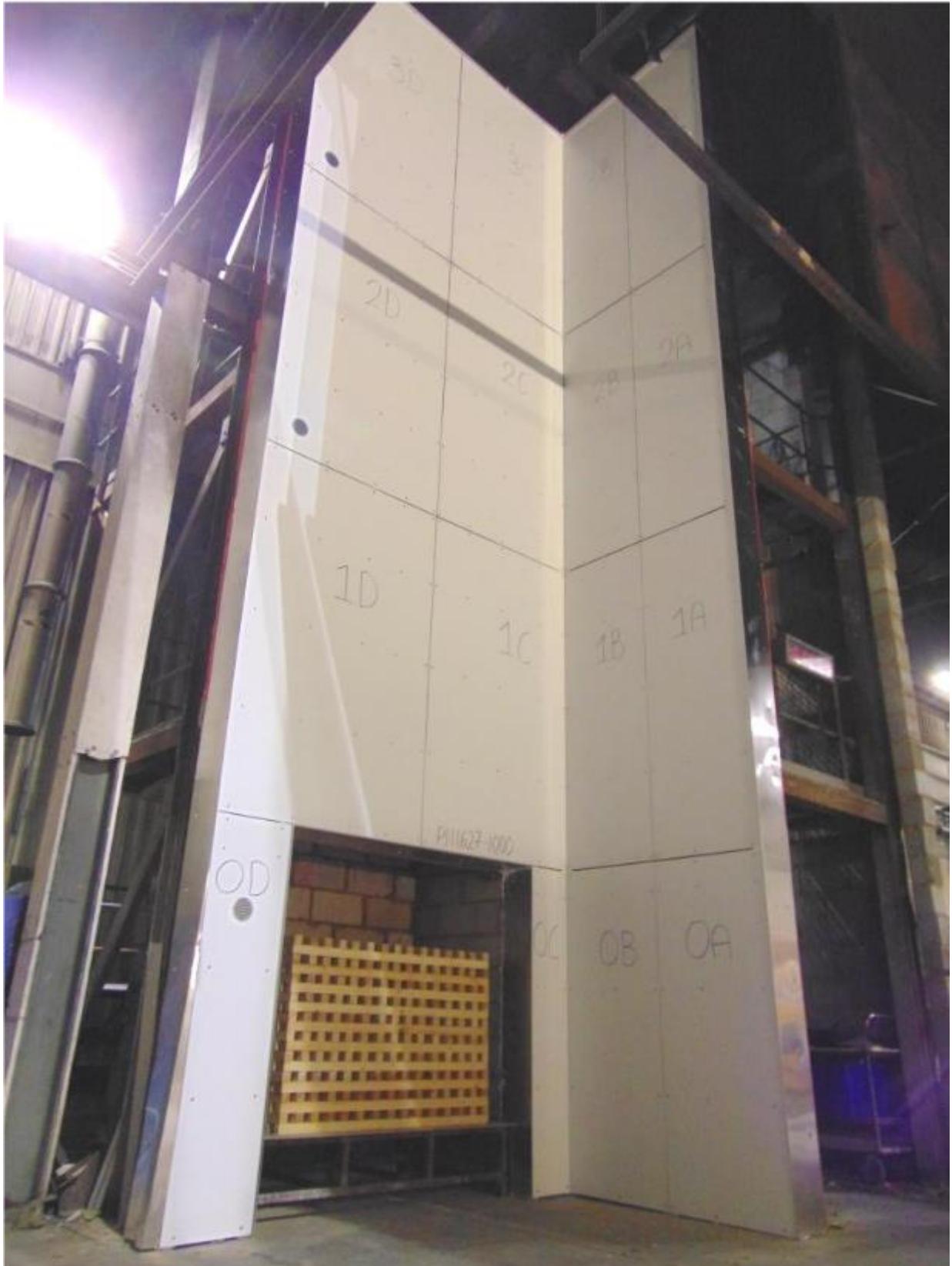
Figure 1. System photos (Main face on the right - Wing face on the left) at the beginning of the test
