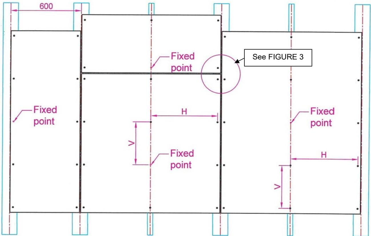
H maximum horizontal distance between fixings  $H \leq 600$  mm
