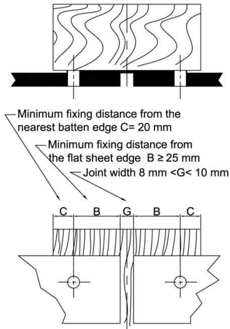
FIGURE 3.b: HOLES DISTANCE FROM SHEET AND METALLIC PROFILE
